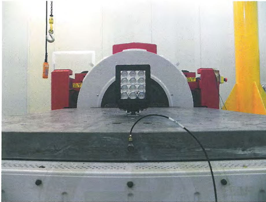
〈Vibration & Shock Test Picture(Front and back:X Axis)〉
