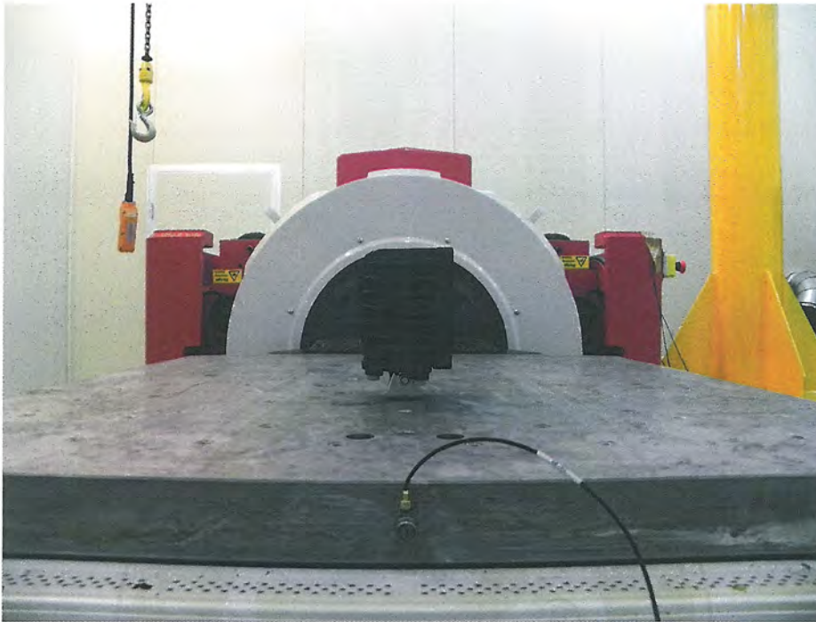
<Vibration & Shock Test Picture(Left and right:Y Axis)>
